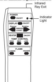
Figure 4 - Remote Control For Electric Fireplace
